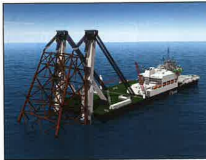
Left to right: Lifting a jacket, tilting it, skid jacket on to Pieter Schelte and sea fasten. International Tug & Salvage, March/April 2011
