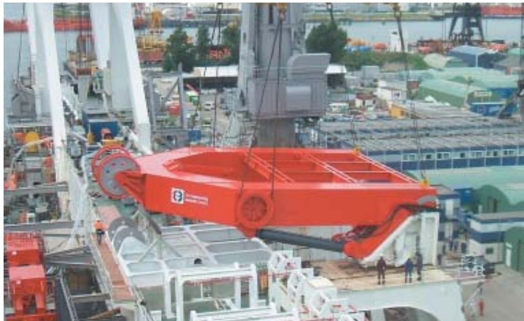
The 550 ton A-frame being placed onboard
