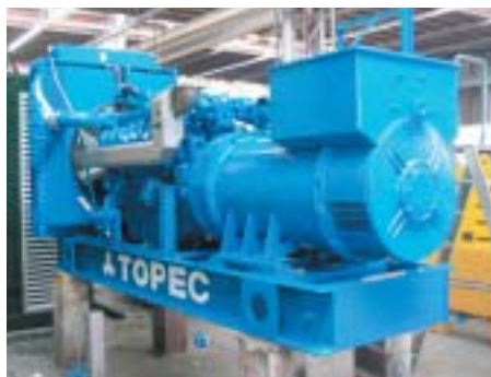
The emergency diesel generator
