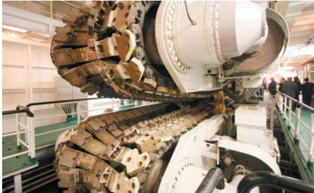
The tensioners keep the pipe stationary and prevent buckling
