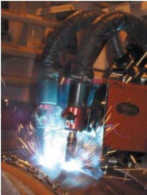
The Phoenix automated welding system
