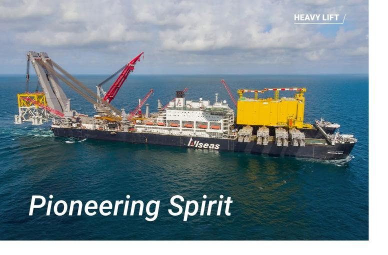
World's largest and most versatile construction vessel, built to transport, install and remove all types of offshore platforms in a single piece.
